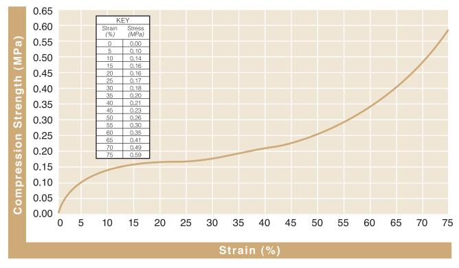
Note: 45 g/l = 2.8 pcf = 20X (g/l = grams per liter; pcf = pounds per cubic foot; X = foam expansion ratio) 1 MPa = 1 N/mm² = 145.04 psi (Units of pressure/stress) Test Speed at 12.5 mm/minute (per ASTM-D3575)
