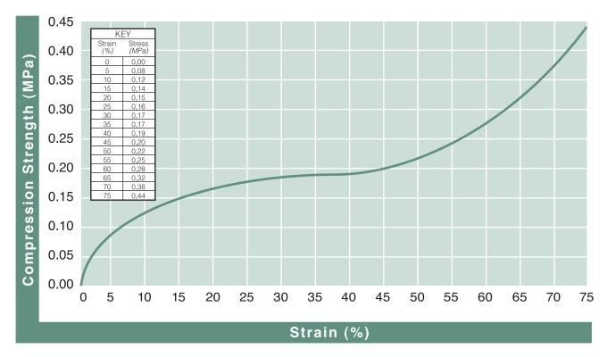
Note: 30 g/l = 1.9 pcf = 30X (g/l = grams per liter; pcf = pounds per cubic foot; X = foam expansion ratio) 1 MPa = 1 N/mm<sup>2</sup> = 145.04 psi (Units of pressure/stress) Test Speed at 12.5 mm/minute (per ASTM-D3575)
