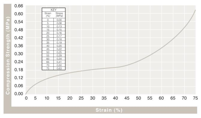
Note: 45 g/l = 2.8 pcf = 20 (g/l = grams per liter; pcf = pounds per cubic foot; X = foam expansion ratio)  $1 \text{ MPa} = 1 \text{ N/mm}^2 = 145.04 \text{ psi (Units of pressure/stress)}$ Test Speed at 12.5 mm/minute (per ASTM-D3575)
